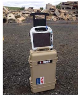
FINDER's microwave radar complements search dogs and sound tools to detect the heartbeats of victims from up to 100 feet away.
