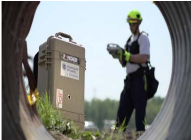
FINDER's microwave radar complements search dogs and sound tools to detect the heartbeats of victims from up to 100 feet away.
